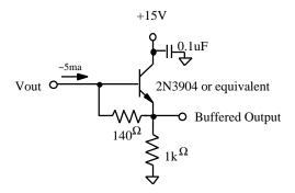
Figure 4 - Recommended Output Structure Load Diagram
