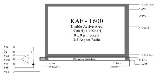
Figure 1 - Functional Block Diagram
