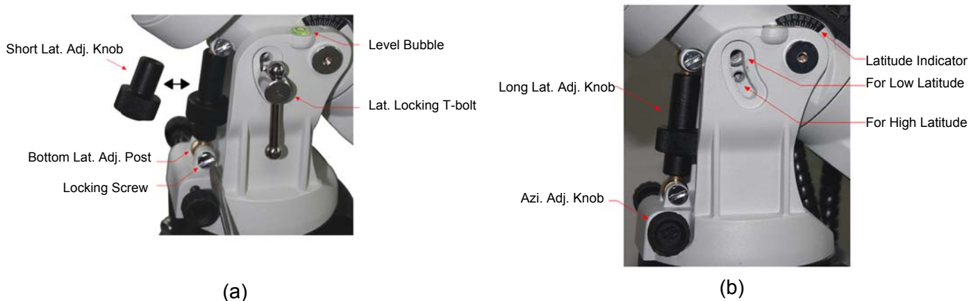
Figure 7. Switching latitude adjustment knob
